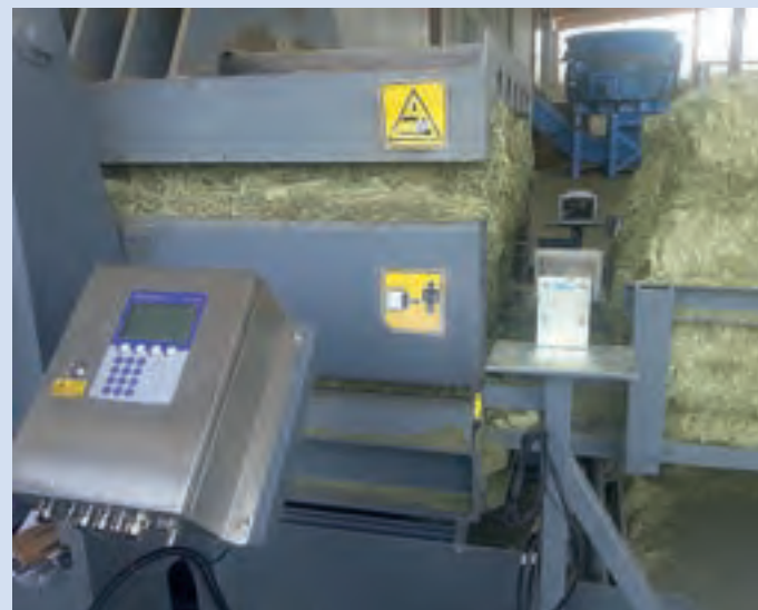
Moisture measurement of bales of straw identification of wet spots – LB 567 with horn antennas.
