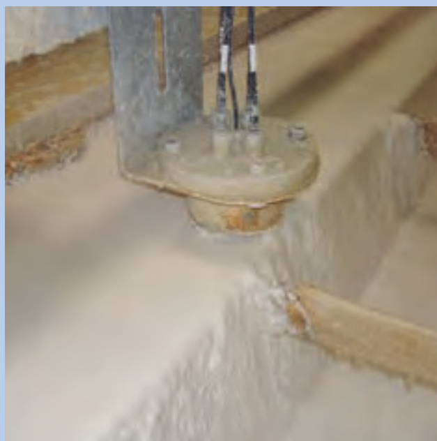
Concentration measurement of milk of lime, installed in a sugar factory – LB 566 with container probe.
