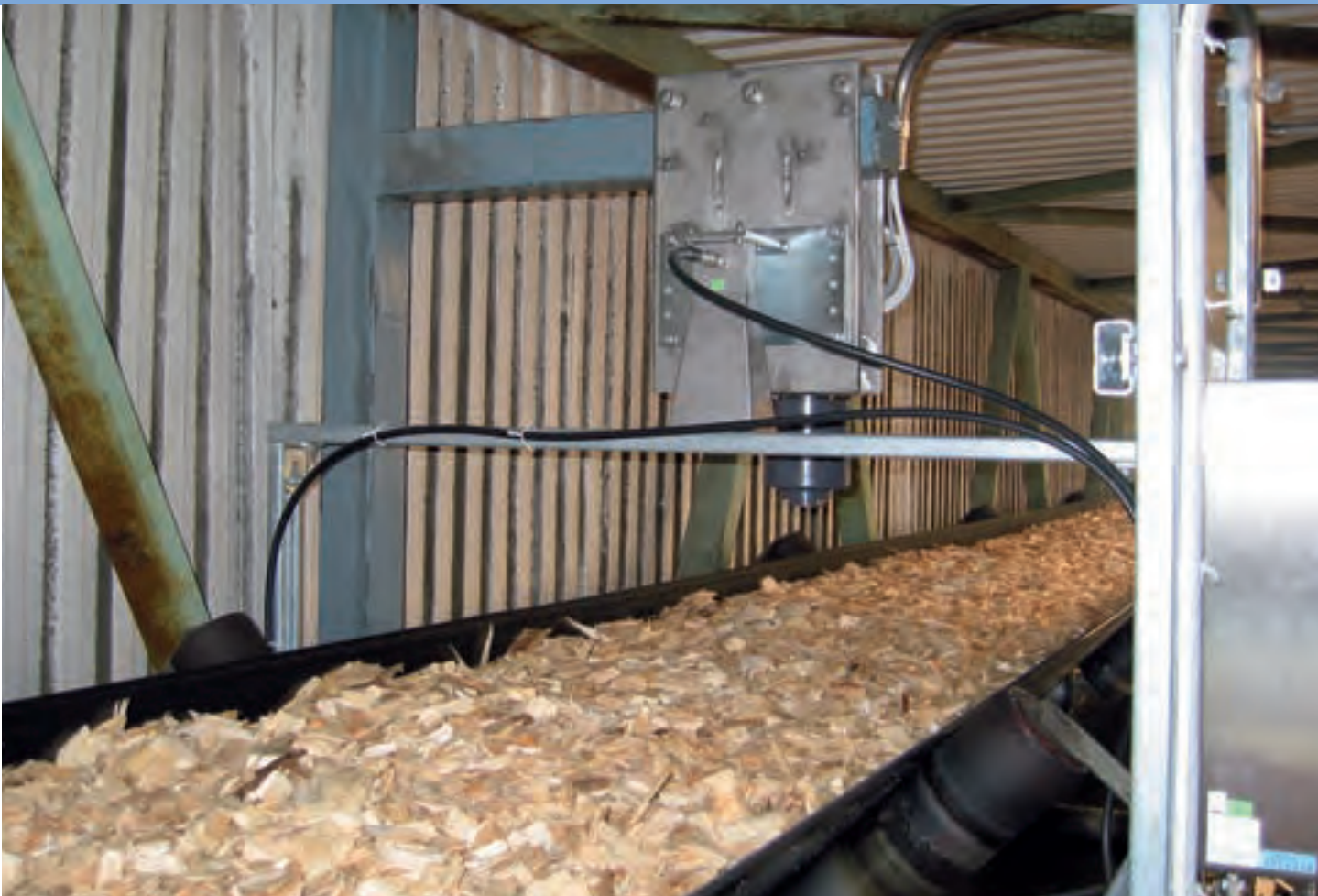
Moisture measurement of wood chips – LB 568 with horn antennas and radiometric area weight compensation.
